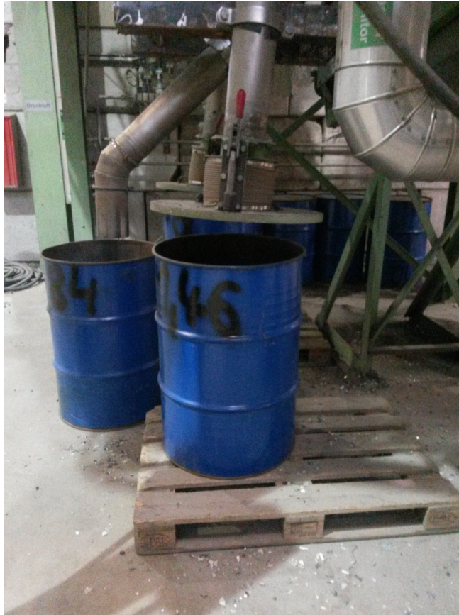
Figure 7 Where the output of the shredder system goes Source: Photo by the author.
