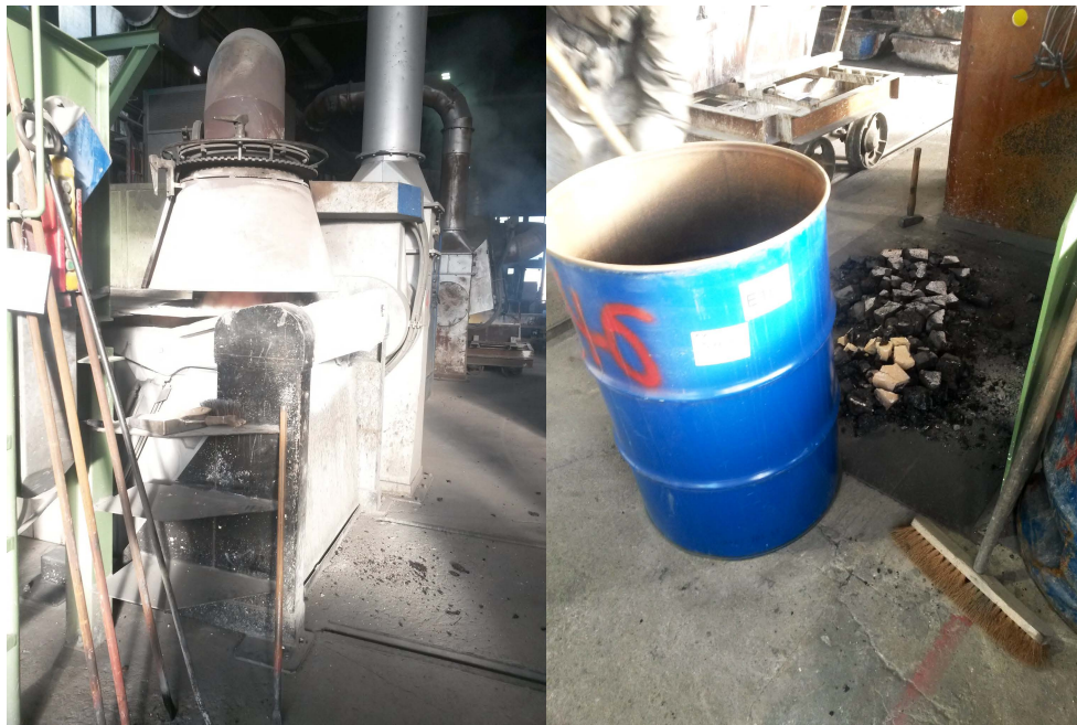
Figure 9 Smelting down the e-waste in a crucible induction furnace (left); and the result of this process (right)
